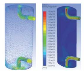
Velocity vector and Velocity contour of flow
